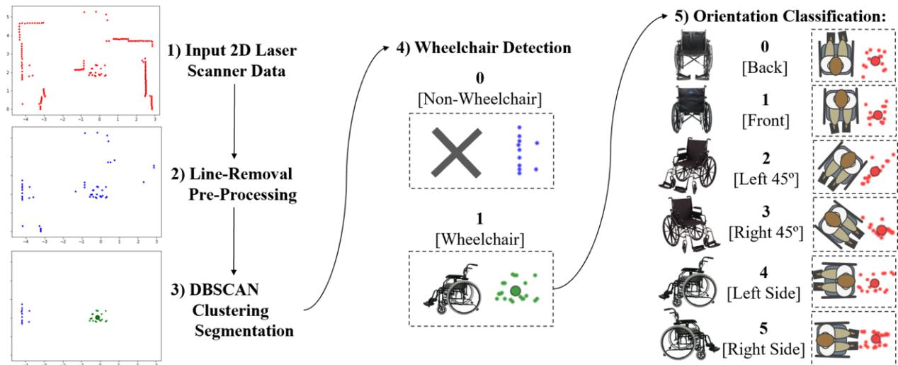
Fig. 1. Overview of the wheelchair orientation estimation algorithm: 1) scan frame of the 2D range data, 2) post-processed data with straight lines removed, 3) DBSCAN segmented, 4) classification on non-wheelchair and wheelchair clusters, and 5) samples of wheelchairs clusters in all orientation classes
