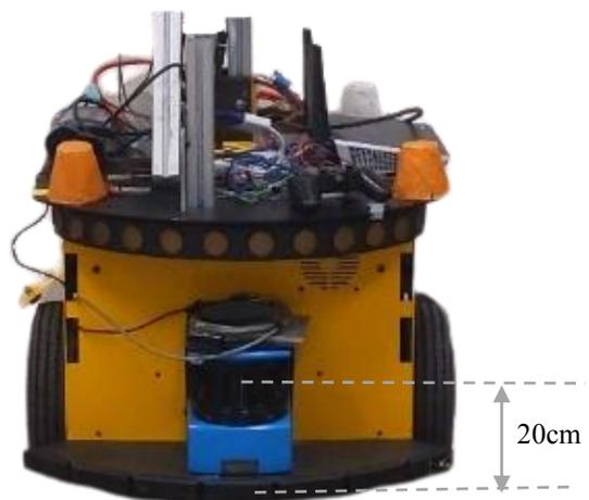
Fig. 2. PowerBot platform with mounted 2D laser scanner
