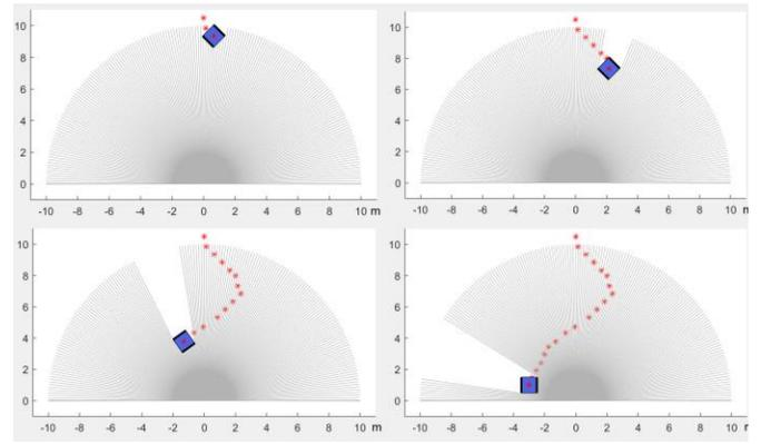
(a) Simulated path of a wheelchair through the laser sensor field
