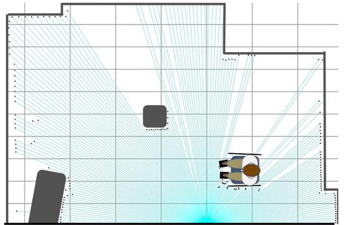
(b) Diagram of the room objects and wheelchair overlaid on range data from the laser sensor
